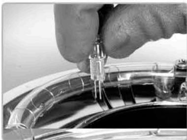
Wearing gloves or using a piece of cloth or tissue, grip the modeling lamp and gently pull it **up and straight out** of the unit. Working with one bulb at a time, repeat this process to remove the remaining seven lamps.
