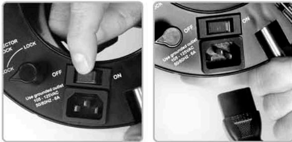
When replacing the modeling lamps, first make sure that the unit is **turned OFF** and that it is **unplugged from the AC power source**. Wait at least five minutes to ensure that the unit does not have any power stored in the capacitors before handling it. You may want to wait longer if you have been actively using the unit.
