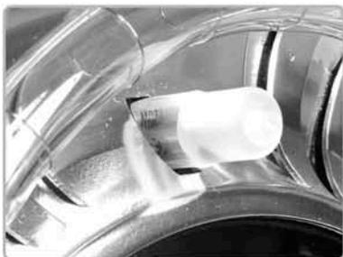
With the new modeling lamps installed, you can plug the unit back into the AC power source and turn it on. If the lamps have been properly replaced, pressing the white **“Model ON”** button on the back control panel of the unit will turn the lamps on. You may then set the lamps to the desired on, off, or track mode and resume shooting.
