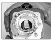
When replacing the flashtubes in your ZEUS flash head, first **ensure that the ZEUS power pack is turned OFF and unplugged** from the AC power source. With the power pack turned off, disconnect your flash head(s) from the power pack and allow the units to cool completely.
