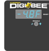
Press the **RECYCLE BUTTON** once to place the flash unit in recycle adjustment mode, then continue to press (tapping, not holding) to cycle through the four recycle indication modes: (1) audible recycle indication, (2) visual recycle indication, (3) BOTH audible and visual recycle indication, or (4) recycle indication off.
