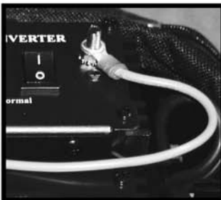
2. attach the wire (then replace wing nut)
